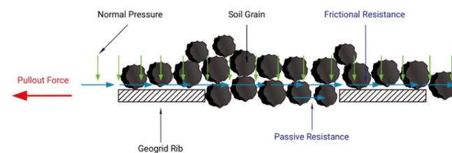
Interaction between the Soil and the Geogrid/Geotextile
